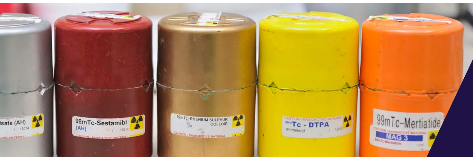
Local shielding of radiopharmaceuticals vials
